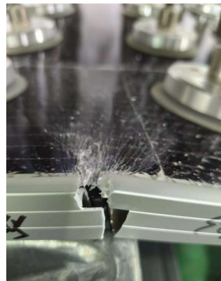
Increased frame and glass breakage was a worrying trend in the 2025 Module Reliability scorecard testing. Image: Kiwa-PVEL
