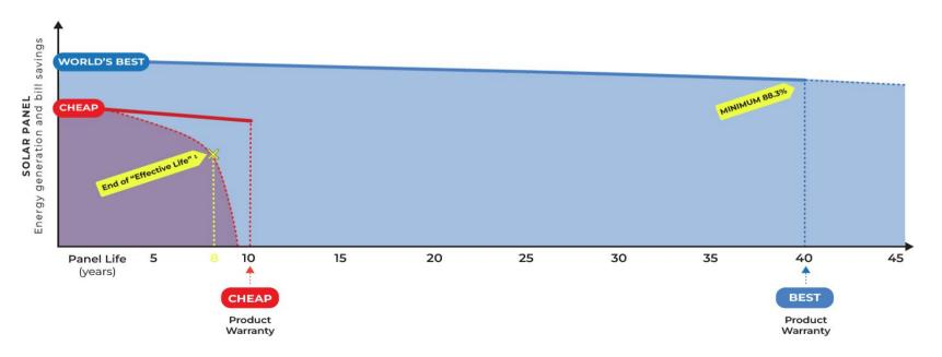
EFFECTIVE LIFE = 70% of panels still generating 70% compared to when first installed.
