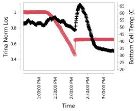
Figure 4.1.4 Overlay of conventional solar panel loss function and bottom row shaded module temperature
