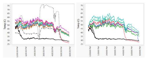
Figure 4.1.5 Module temperature trends for P-Series (left) and conventional solar panel (right) in portrait
