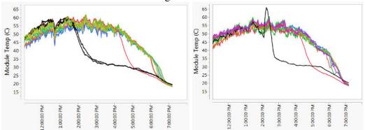
Figure 4.1.3 Module temperature trends for P-Series (left) and conventional solar panel (right) in landscape
