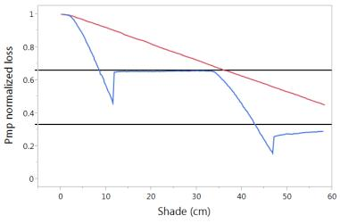
Figure 4.1.1 Normalized loss function in landscape, P-Series (red) and conventional solar panel (blue)
