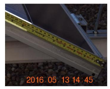
Figure 3.2.3. Shade length on a P-Series module as measured on 5/13/16.
