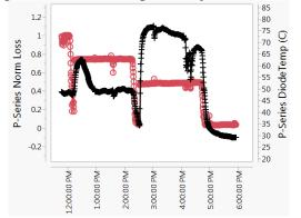
Figure 4.1.6 P-Series loss function (red) and bypass diode temperature (black) in portrait
