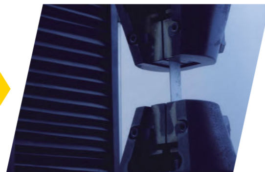
Anti-pull force testing
