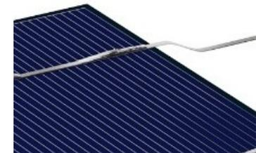
Conventional panels connect cells with soldered ribbons - these fatigue, causing hotspots and power loss
